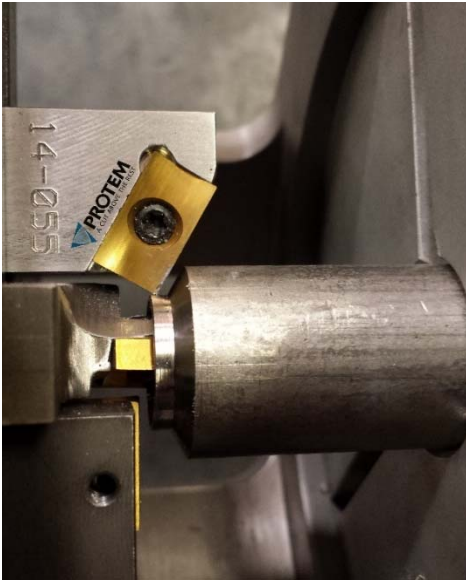
Figure 6 J bevel performed on a tube from superduplex, wall thickness < 20mm with an od clamping beveling machine PROTEM SE90NG
