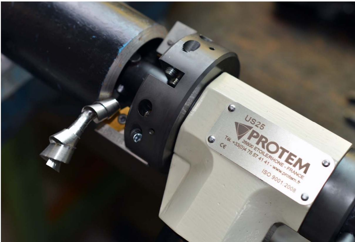
Figure 5 V bevel performed with a PROTEM US25
