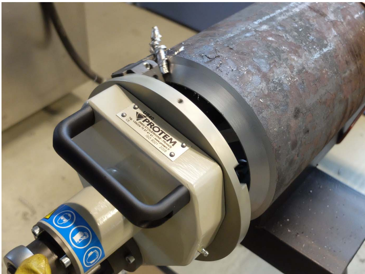
Figure 16 Pipe Beveler with axial stroke PROTEM US40
