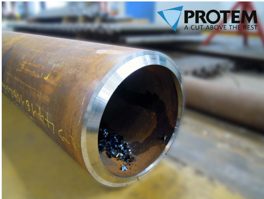
Figure 8 Compound bevel made with a high speed beveling bench PROTEM BB3-16
